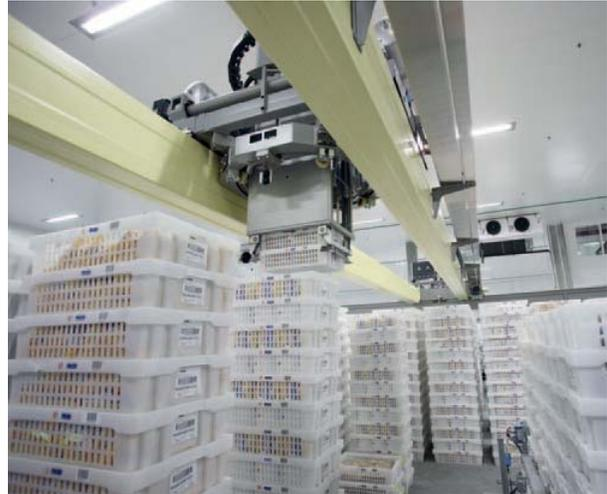
Gantry robot operating stack buffer
